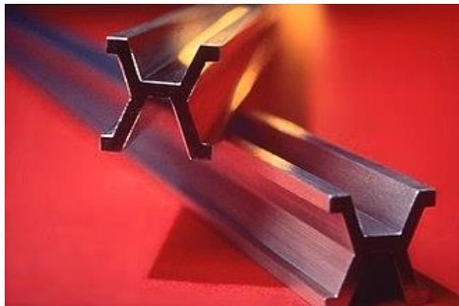
Historical international prototype of the metre, made of an alloy of platinum and iridium, that was the standard from **1889 to 1960**
